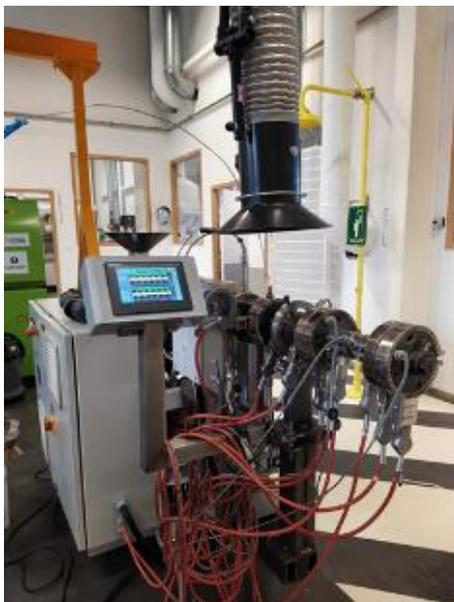
*Figure 6: Single screw extruder (CANOE) equipped with supercritic CO2 pump*
