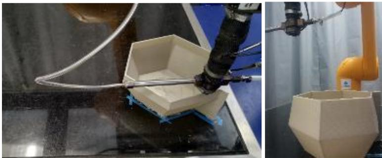
*Figure 5: Vase printed from pellets by 6-axis robotic arm (CANOE development)*
