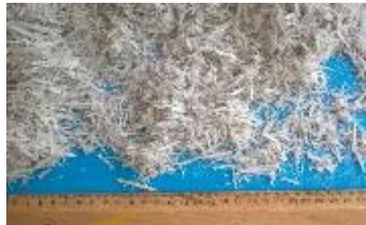
*Figure 1: A wind turbine blade made with glass fibers infused Elium® - Grinded scraps*
