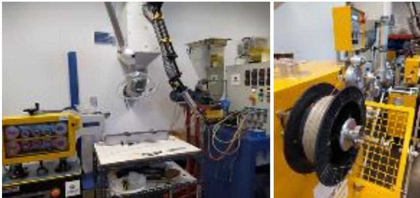
Figure 3: 3D filament production – Spooling (CANOE Development)
