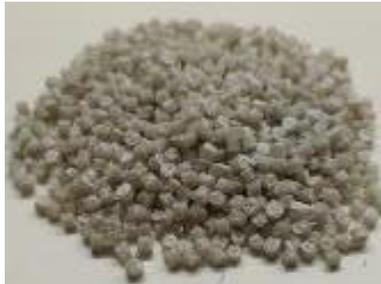
Figure 2: PMMA/Elium®/FV pellets
